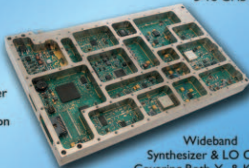
Amplified Switch Filter Bank 9 Selectable Bands 5-18 GHz
