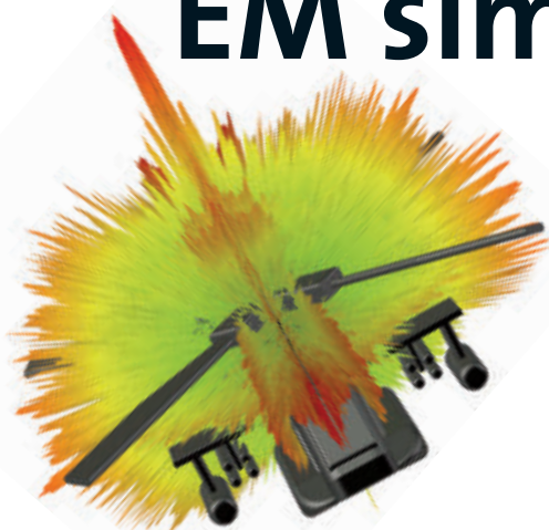
RCS & Surface Current Simulation of a Helicopter
